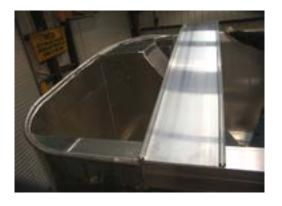
1A: Placement of master bow is dependent on depth of cap or bonnet to be installed. In most cases it should be a max of 24".
