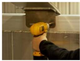
3D. Align leg holes with marks, drill and secure bow legs with 3/8" machine bolts provided.
