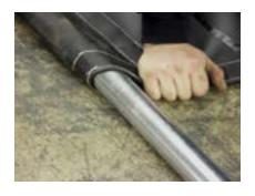
6D: Insert the 2" roll pipe open end first into pocket from rear of tarp and slide through to other end. Leave 18" (length varies) of splined end out at rear of tarp.
