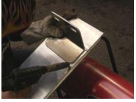
1C: Place bow legs flush on master bow at marks and weld in place (both sides).
