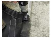
6E: Fasten tarp to roll pipe at rear with "U" clamp and 1/4" tek screws provided. Install "U" clamps one on every seam apart down the length of tarp.
