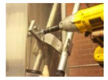
With tarp in locked position, pull crank down and in against the side of trailer. Mark the "J" hook position. Install "J" hooks with the 3/8" machine bolts provided.
