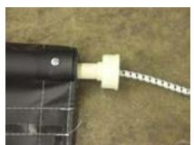
6G: Install Roll Return tube in front of roll pipe. Tap plastic flange until flush with end of roll pipe.
