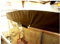
3B: Work bonnet over front of bulkhead. Align seam with top weld, do not let seam ride over front of bulkhead.
