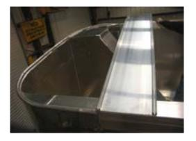
1A: Placement of master bow is dependent on depth of cap or bonnet to be installed. In most cases it should be a max of 24".
