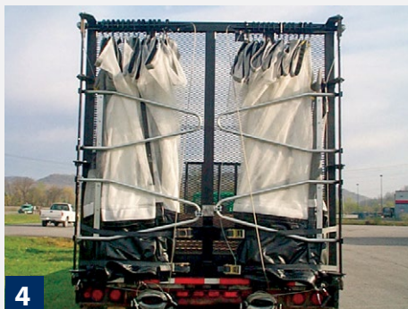
(1) Airbag material is reinforced with vinyl and steel cables (2) Electric motor option raises and lowers the main cable (3) Steel bearing rollers for smooth operation (4) Hoops lock the tarp compactly out of the way (5) Manual winch option
