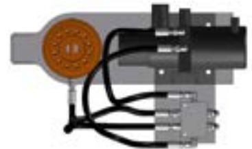
Figure 7 -Final Assembly of Hoses
